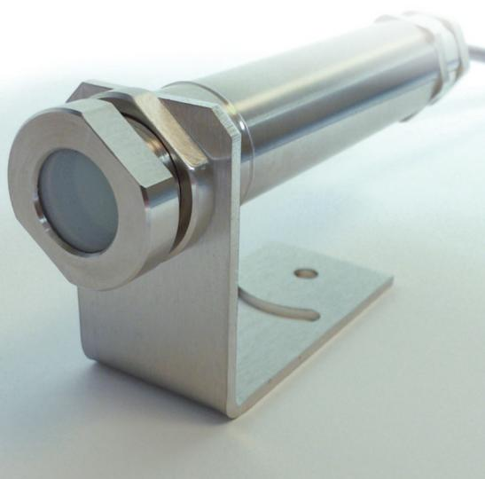
The protective plastic window models PWS and PWL are designed to help protect the silicon lens of Calex infrared temperature sensors from mechanical damage, and to help retain fragments of the lens if it is damaged. This is the preferred window material for food and pharmaceutical industries.
