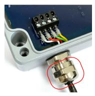
With power off, fully unscrew the outer nut of the cable gland on the electronics module.
