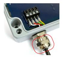
With power off, fully unscrew the outer nut of the cable gland on the electronics module.
