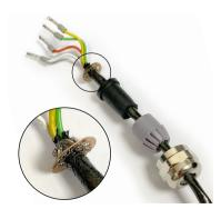
Ensure the cable shield braid is folded back over the cable jacket and gripped by the metal shield ring. This ensures a good electrical connection to the cable gland.
