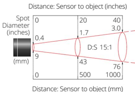
The sensor may be used at longer distances than shown, and will measure a larger spot. The measurement accuracy is not affected by the measurement distance.
