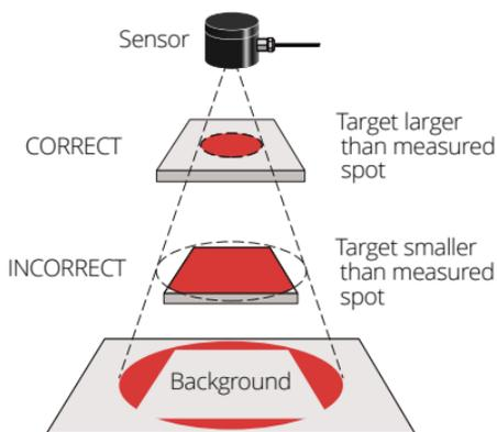
We normally recommend that the target should be at least twice the size of the measured spot for maximum accuracy.
