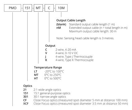
**PMO** PyroMini OEM infrared temperature sensor with miniature sensing head and separate electronics module
