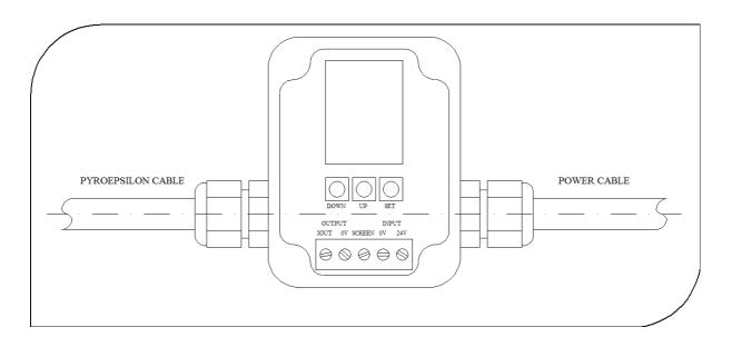
Note: The output of the PyroTune is isolated from the power supply input for up to 1kV
