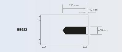
The BB982 Portable Blackbody Calibration Source allows for calibration of non-contact infrared thermometers over the temperature range -20°C to 125°C.
