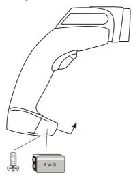
To prevent data losses, the battery change should only be done if the instrument is not working.
