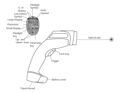
Pull the trigger to switch on the instrument. This is a two stage trigger. To lock the trigger for continuous readings, pull the trigger fully back and push up the lock-key.
