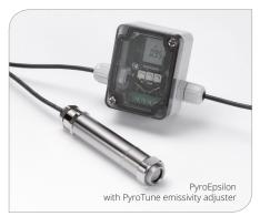
The **PyroEpsilon** is a simple infrared temperature sensor with an adjustable emissivity setting. It is ideal if the target is partially reflective.
