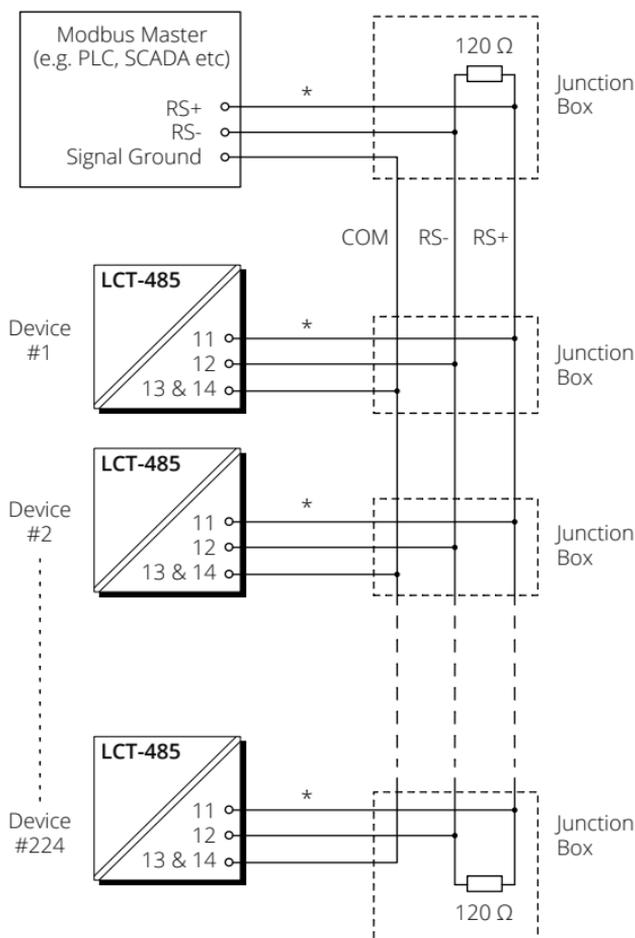
\* Ensure the distance between each device and the network bus is as short as possible.
