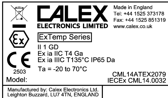
Figure 2: ATEX/IECEx marking on the ExTemp.
