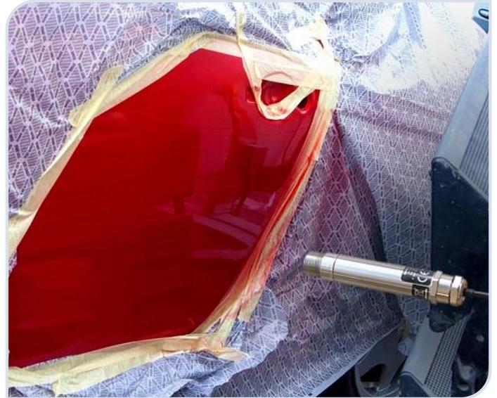
The Calex sensors allowed direct, accurate, on-line measurement of the surface temperature. The infrared sensor also allowed separate controls to be introduced for top and side heating. This was valuable, due to the differing thermal masses and therefore heating rates of the automobile roof and sides.
