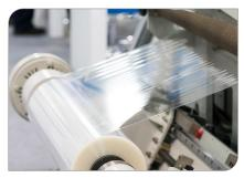
Transmissive materials are difficult to measure. A specialised sensor such as the PyroCube P may be required to achieve a good reading.
