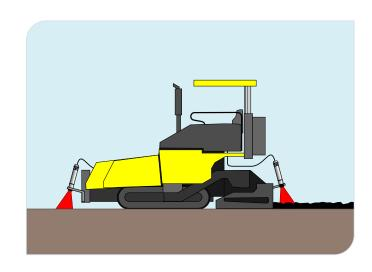
Two model PC151MT-0 sensors are mounted on the paver and aimed at the road surface, before and after laying the tarmac. A sensor can also be placed on the roller to monitor the tarmac temperature immediately before it is compacted.
